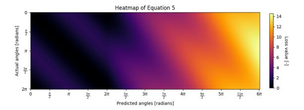
Figure 5: Heatmap of Equation 5 for angles (in radians) in the range of  $[0, 2\pi]$  on the y-axis and angles (in radians) in the range  $[0, 6\pi]$ . The bar on the right indicates the values corresponding to the colours.
