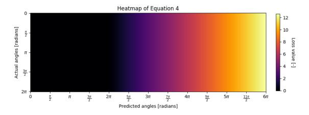
Figure 4: Heatmap of Equation 4 for angles (in radians) in the range of  $[0, 2\pi]$  on the y-axis and angles (in radians) in the range  $[0, 6\pi]$ . The bar on the right indicates the values corresponding to the colours.
