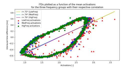
Figure 6: The ITDs (y-axis) correlated with the activations of the neural network (x-axis) for the three frequency categories. \* indicates significance at p < 0.001.
