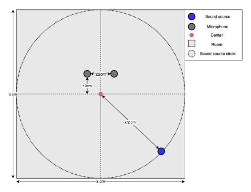
Figure 1: An exemplary environment with sound source. The legend is given in the top-right and the (0, 0) coordinate is in the top-left.
