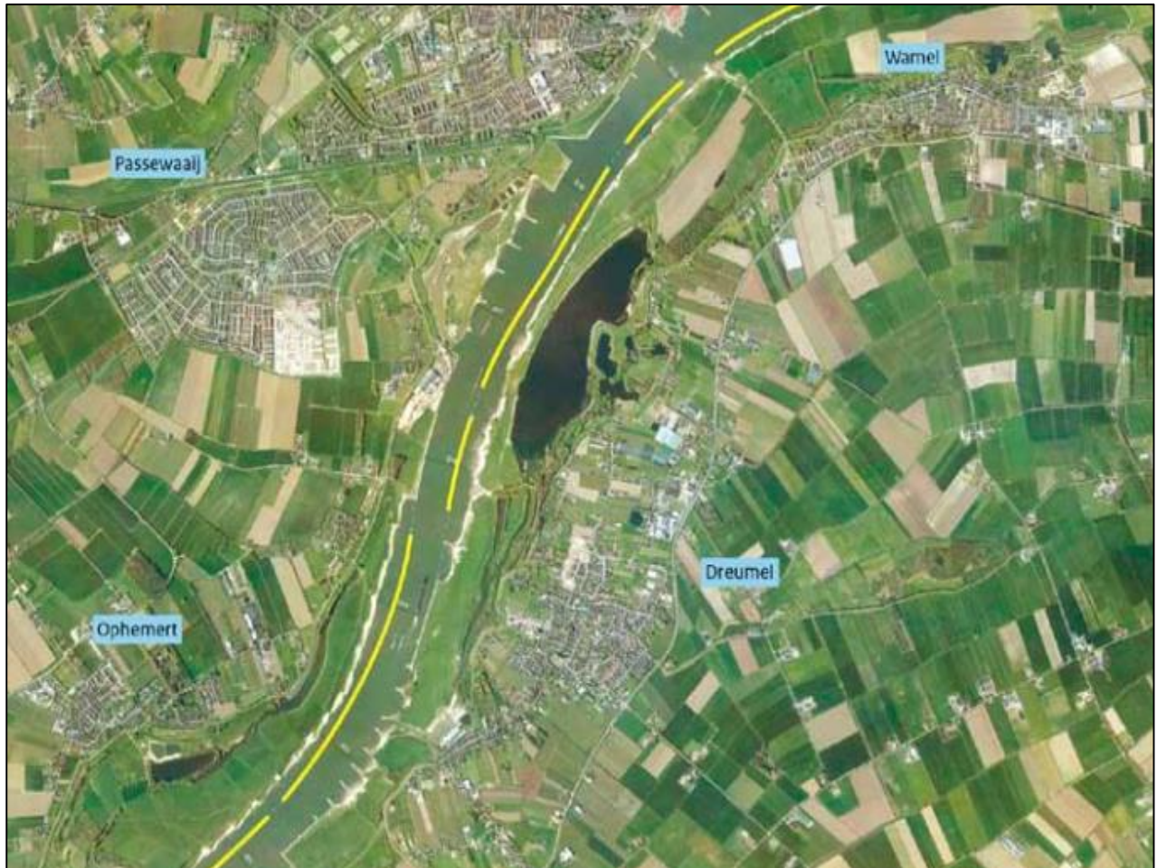
Figure 1.3: Map of the project location and the intended measures. Note that the groynes in the outer river bend will remain, while the longitudinal dams are placed along the inner bend (Rijkswaterstaat, 2012)
