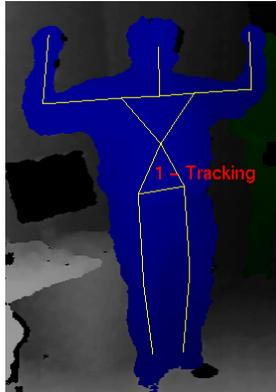
**Figure 5.1:** The psi pose needed to calibrate the body pose tracker.
