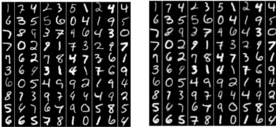
Figure 4.11: Original Images (left) and reconstructed images (right) with latent space of 8 dimensions
