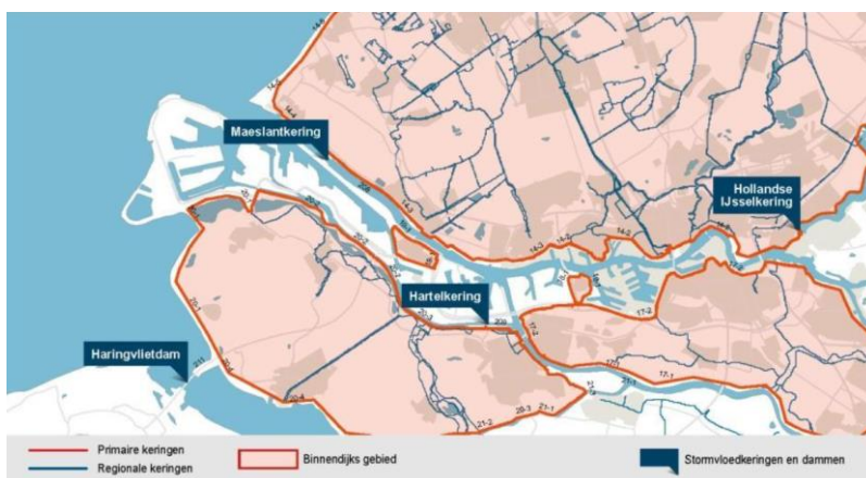
Figure 17: Structural flood defence system Rotterdam (Municipality of Rotterdam, n.d.-c)
