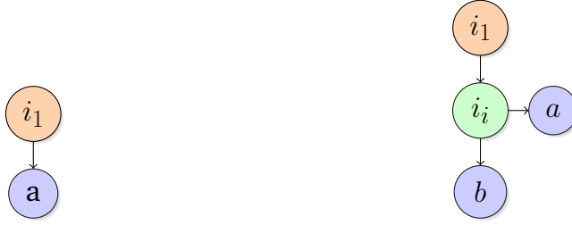
(a) A toolbox which always performs action a , no matter what the situation is. (b) A toolbox which performs action a in all situations where i_i is true and b in all situations where i_i is false.
