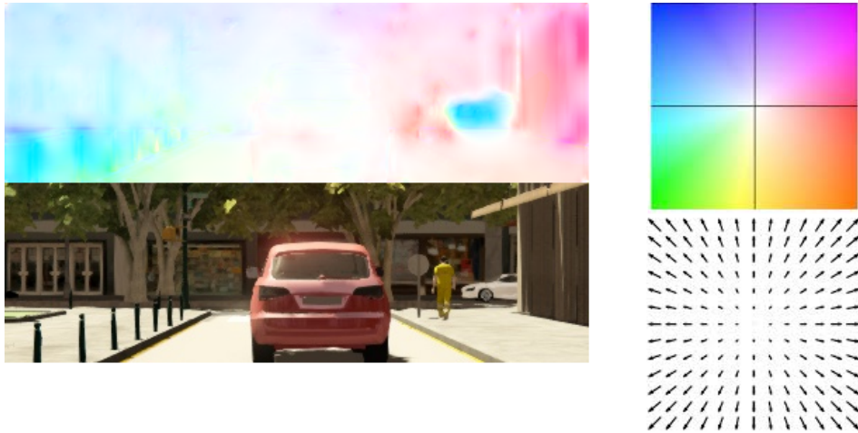
Figure 3.1: An example of a dense flow representation using colours to indicate the vector. On the right is a legend of the colour coding.[5]
