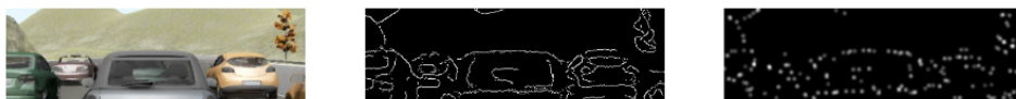
Figure 2.1: An example of simulated phosphene vision. From left to right: The raw image, the edges in the image, the phosphene image.
