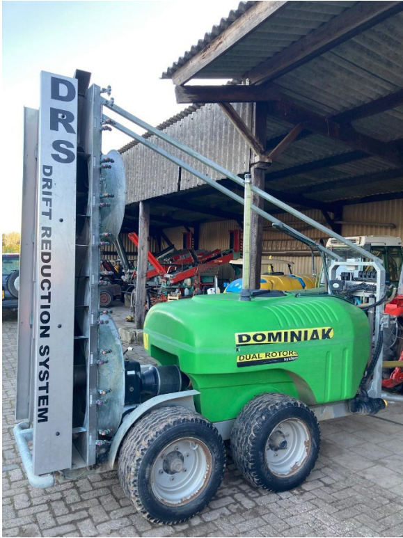
Image 4 Crop protection sprayer with drift reduction in a shed
