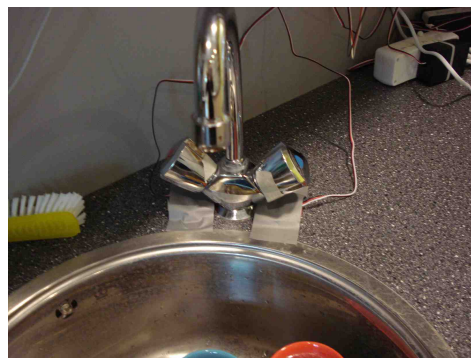
Figure 3.6: Magnet contact sensors used to measure twisting of the watertaps
