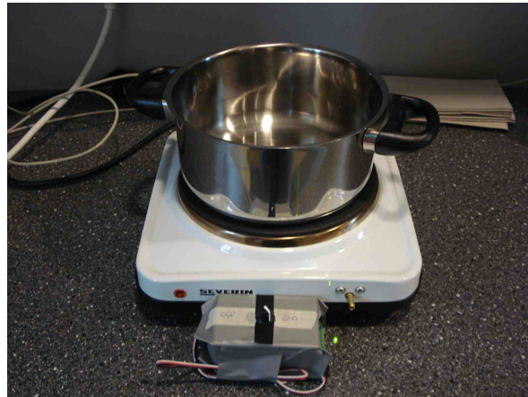
Figure 3.8: Rotation sensor attached to the interfacekit and the cooker
