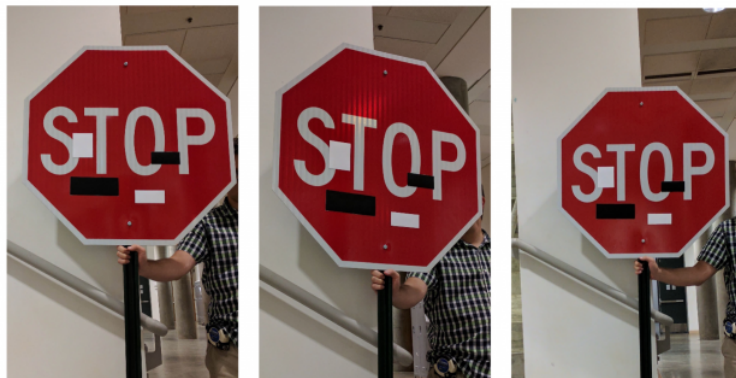
Figure 1.1: Stop sign modified with black and white stickers. Used for adversarial attacks by researchers from Washington University [1].
