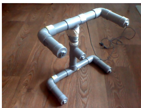
Figure 9: Picture of the rigging. It has 4 targets and a central button and is made from a disassembled computer mouse, buttons and piping used for plumbing.
