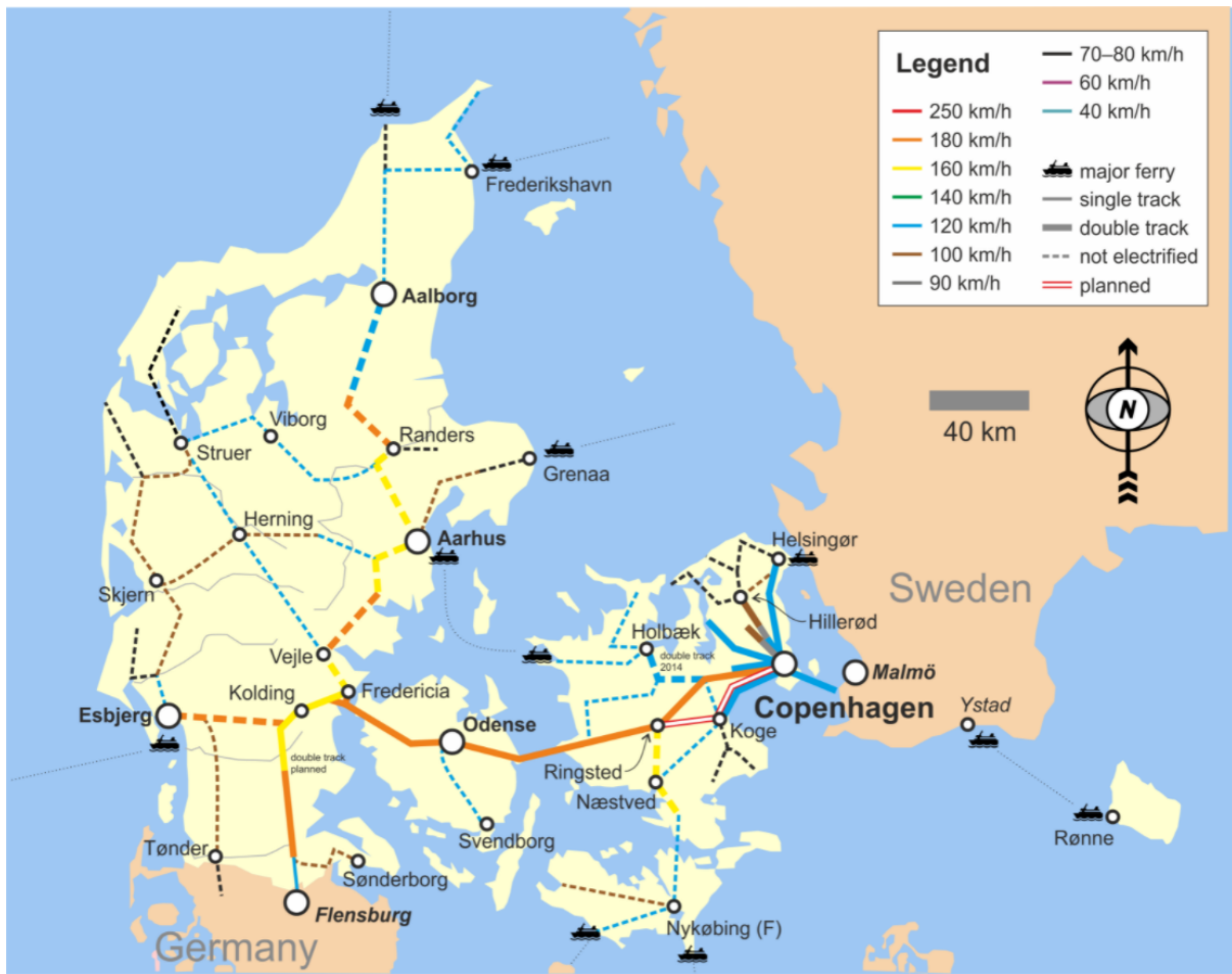
Afbeelding 1.3: Maximum speed on the Danish railways, as of 2014 (Creative Commons - Wikipedia, Classical geographer & Kopiersperre, 2014a).
