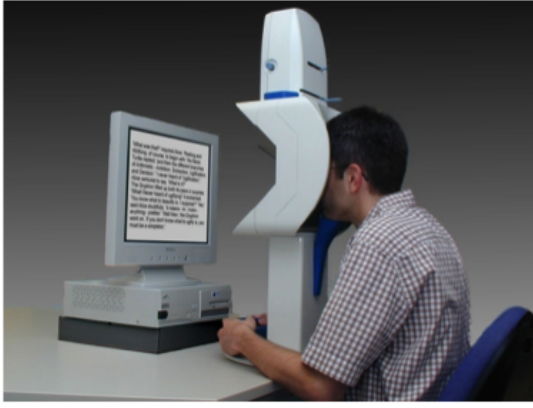
Fig. 1. The iView X'Hi-speed: a desk mounted eye tracker. During use the subject rests their chin on the support, to minimize head movements.
