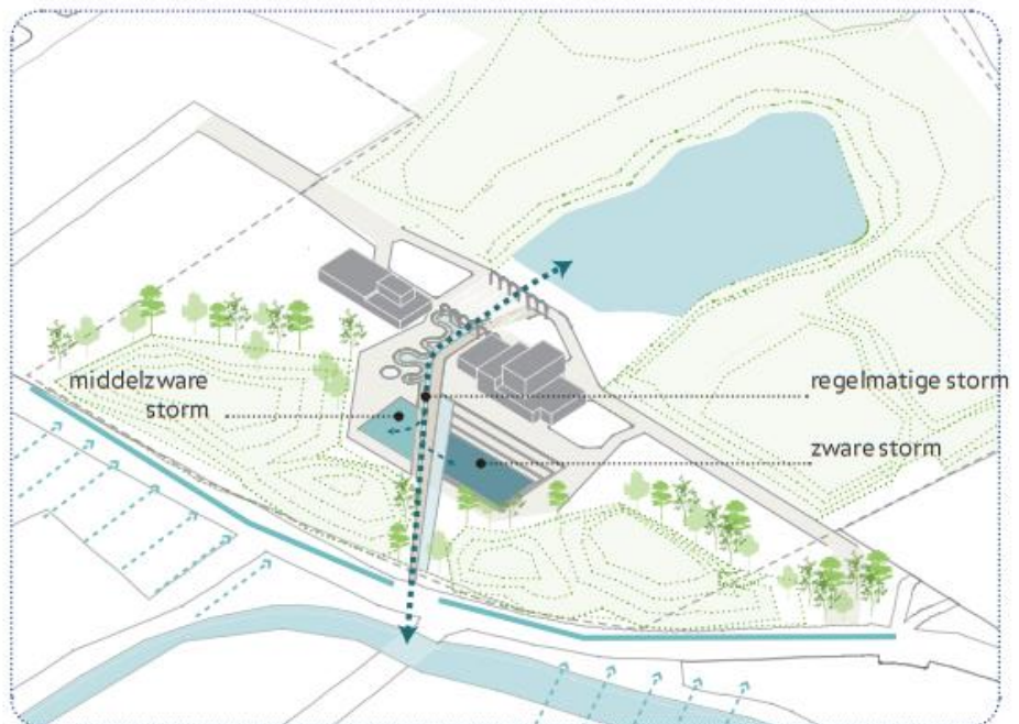
Figure 20. Planned situation in Park de Valkenier: function of the water square before and after a period of rainfall
