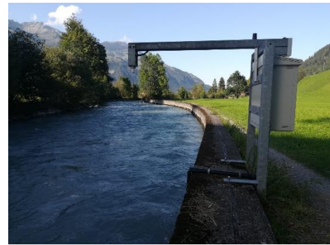
Figure 7: Water Level Measuring Device near Kandergrund (Own Observation 15-09-2019)
