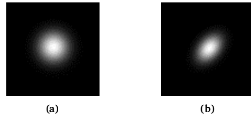
Figure 6: Phosphenes are shown as either (a) a circular dot, the brightness of which is given by a Gaussian distribution or (b) a Gabor filtered version of the Gaussian blob, with a random orientation.
