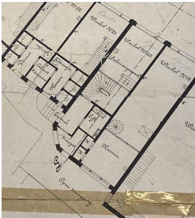
Preliminary plans for 'Cabinets d'Aisance' (public bathrooms) behind stores no.21 & no.22 ('open doorgang' was the passageway from the not-yet-built third arm to these rooms)
