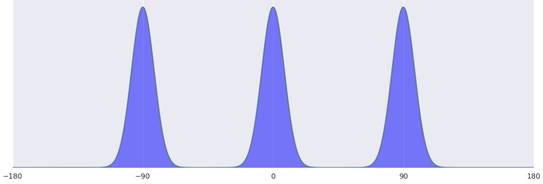
Figure D.2.1: Multi-modal distribution on the orientation between steps. In our model we favour straight paths and turns.
