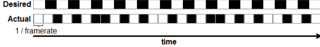
Figure 4.3: The difference between which states (black and white) are desired at each point in time and which states can actually be rendered. The length of each rendering alternates between being too long or too short, but is never quite correct. The example shown was derived from a 60 Hz device trying to render 24 Hz stimulation over the course of a half second.
