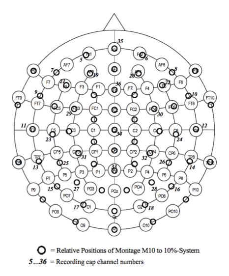
Figure 2: Detailed view on the positions of the electrodes in the electrode cap placed on the scalp according to the M10 system. The electrodes that are used are marked with a black circle and a number from 5 to 36.
