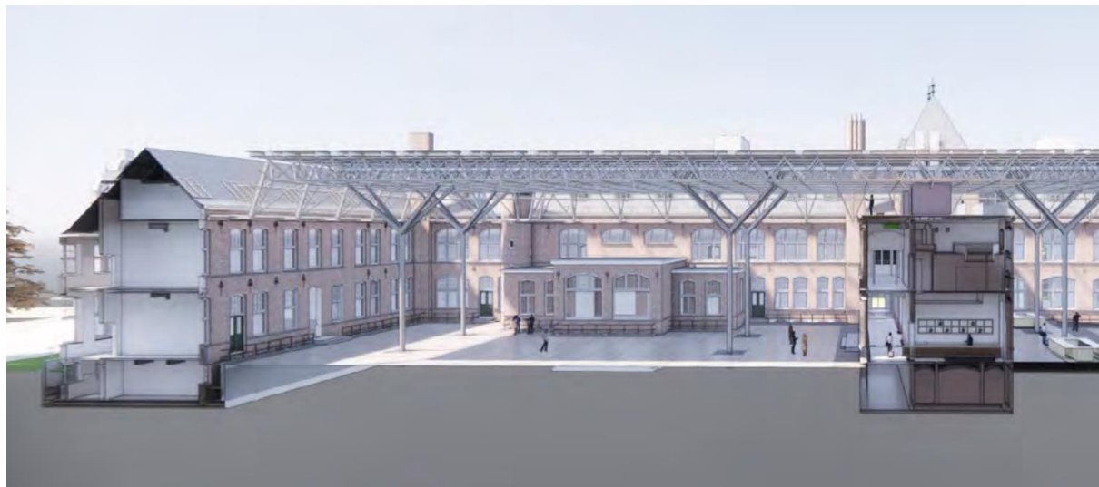
Figure 27: Cross section image of the roof covering the courtyard, retrieved from (Vlerken, 2023).
