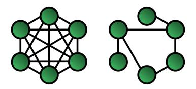
Figure 17: A mesh network is often not fully (left) but only partially connected (right). (Source: GW Simulations / Wikimedia Commons / Public Domain)
