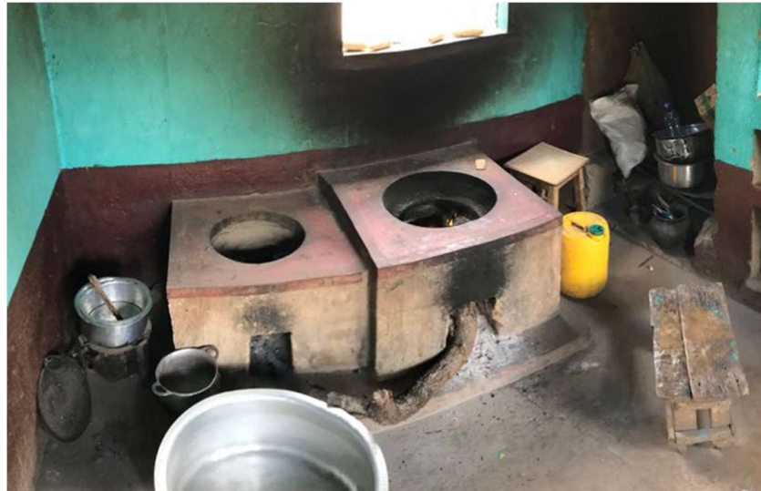
An improved firewood stove (Rocket Stove) in Kitui, Kenya. Source: Own image
