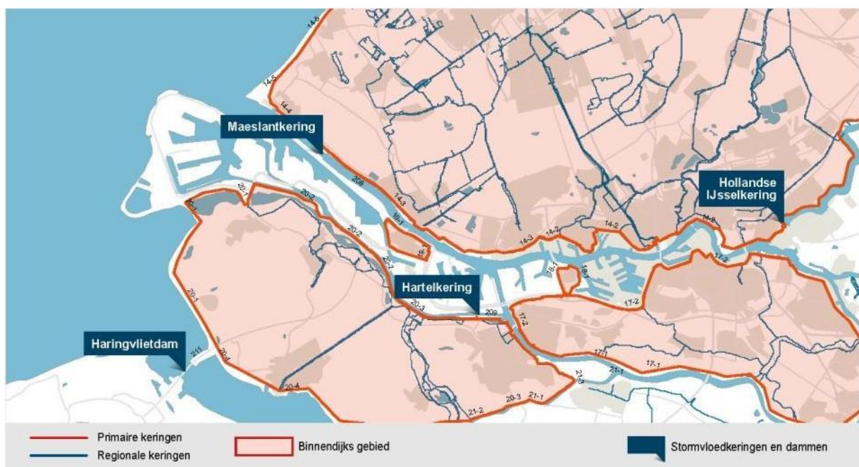
Figure 13: Water barriers around Rotterdam (Gemeente Rotterdam, n.d.)
