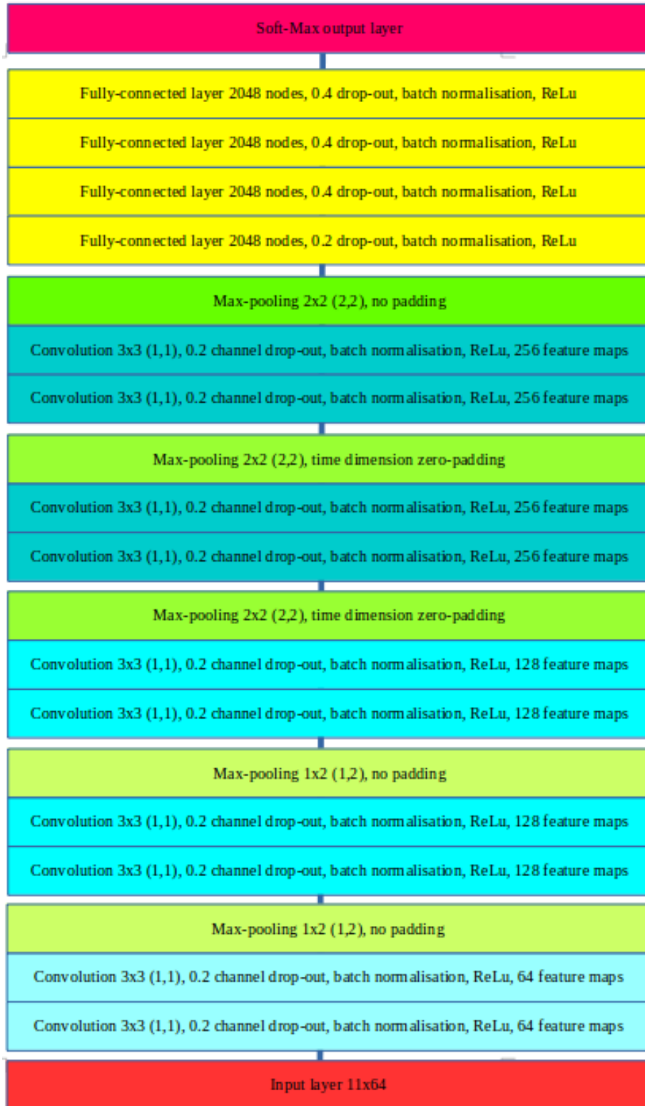
Figure 11: Overview of the DNN architecture used in this project.
