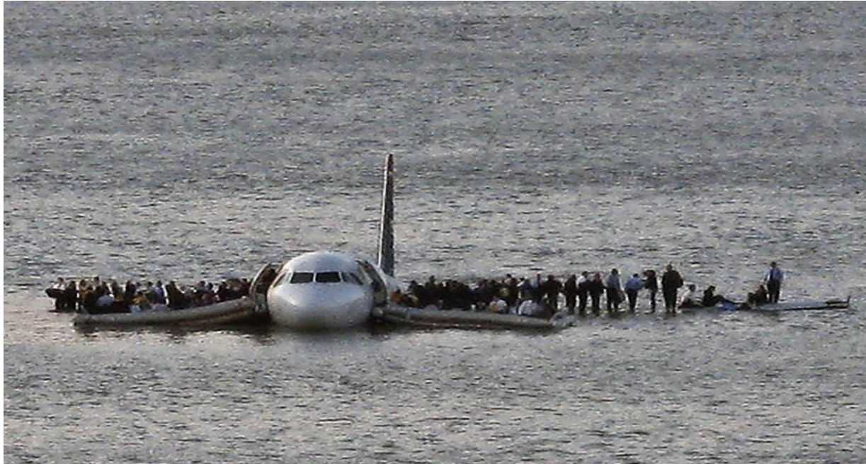
Figure 7. Aeroplane occupants on the wings and in the slide/rafts after the evacuation.
