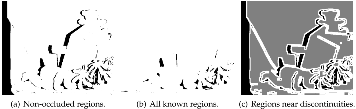
Figure B.1: An example of different image region subdivisions for the evaluation of stereo algorithms (using the “teddy” image). For each figure holds: errors are only evaluated in the white regions. Figure B.1(a) shows non-occluded regions (white) and occluded and unknown regions (black). The second Figure B.1(b) shows all known (including half-occluded) regions (white) and unknown regions (black). Figure B.1(c) , finally, shows regions near depth discontinuities (white), occluded and unknown regions (black), and other regions (gray).
