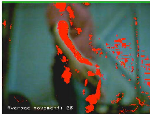
Figure 4.2: Motion detected when walking past the camera
